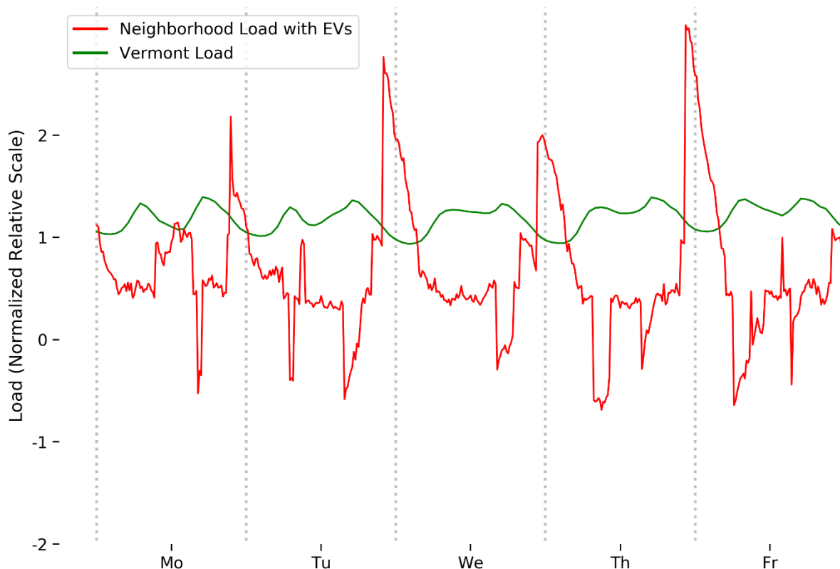
Figure 6. Simulated normalized neighborhood load with widespread EV adoption vs. Vermont actual 2021 load during the cold weather high grid stress week.
