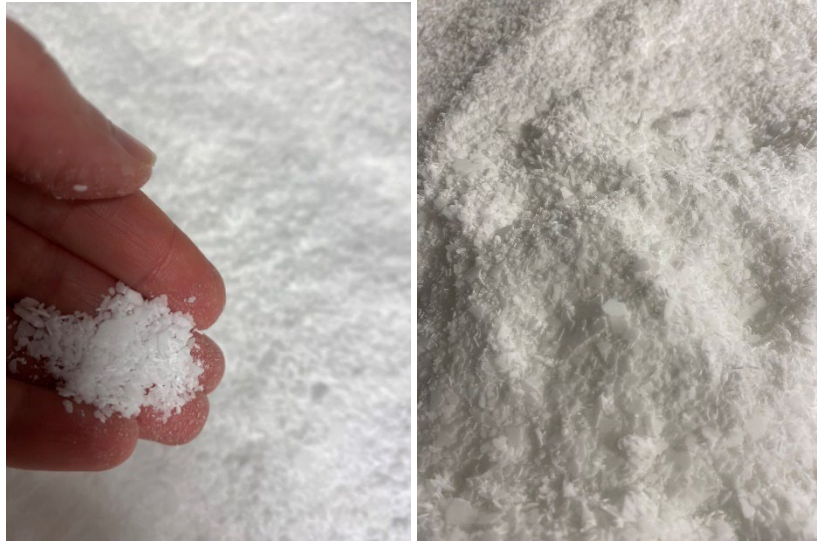
Image 4. PCM is a granular wax and has the feel and consistency of shredded crayons. Upon solidifying after the first melt, the material appears as a solid block.
