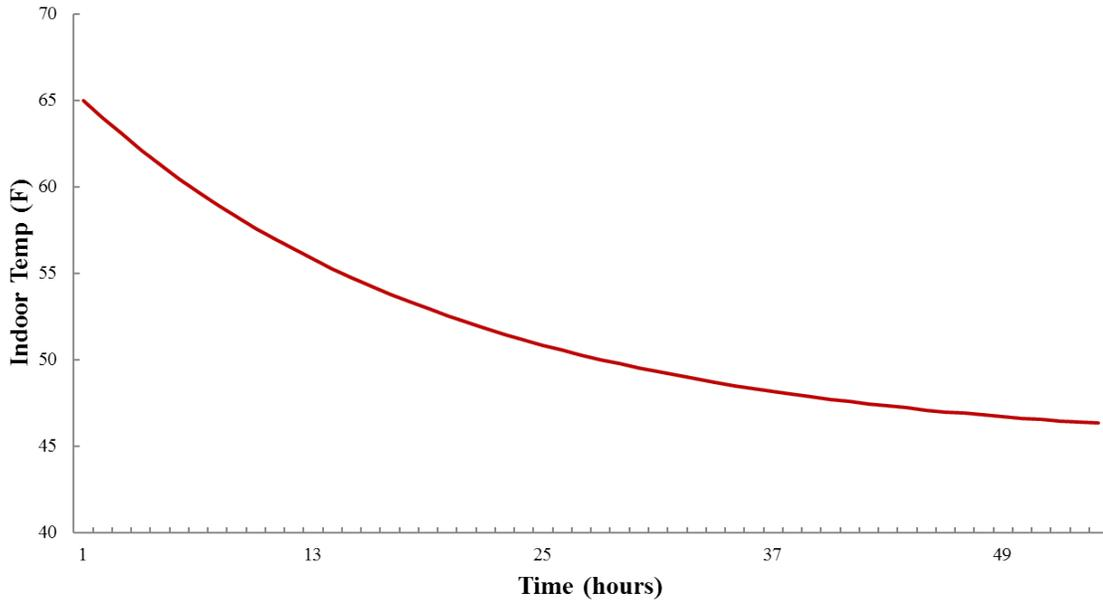
**Figure 1: A simplified model of indoor heat loss based on (specific heat of air \* volume \* density) + internal loads – (air infiltration + ventilation)**
