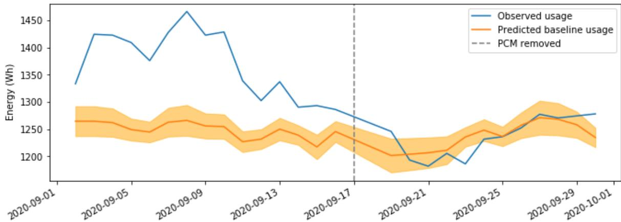
Figure 2. Chest freezer observed energy use with and without PCM, compared to baseline model prediction of an empty freezer with a 95% confidence interval.
