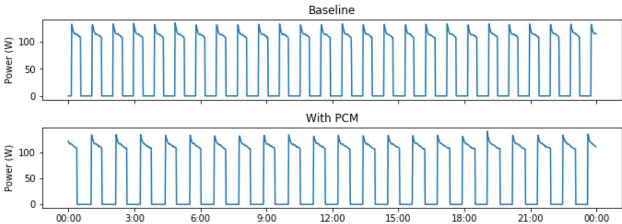
Figure 3. Comparison of chest freezer compressor cycles without PCM (Baseline) and with PCM, across a 24-hour period.
