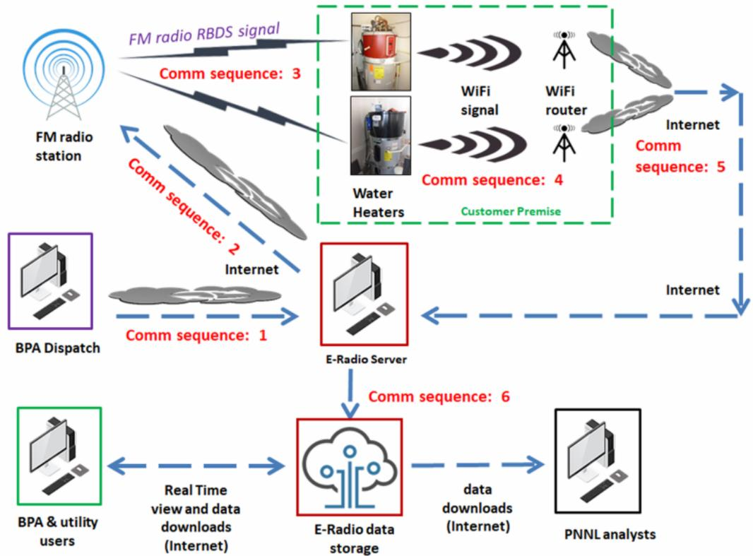
Figure 1. Example of communications pathways, demonstrating an analogy for handling flexible load management.
