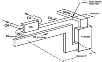
**Method 4: "Return-return"** | Fresh air leaving H/ERV is injected into return side of the furnace ductwork AND exhaust air returning to H/ERV is drawn out from return side of furnace at a point at least 3' upstream of the fresh air injection.
