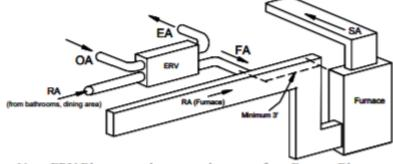
Note: ERV Blower may be operated separate from Furnace Blower
