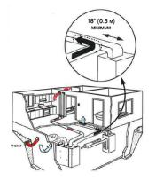
**Method 3: "Return-supply"** | Fresh air leaving H/ERV is injected into supply side of the furnace ductwork AND exhaust air returning to H/ERV is drawn out from return side of furnace.
