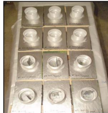
1-3 Flat head screw with sealant
