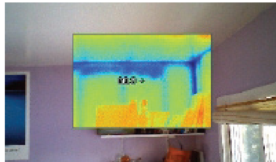
Figure 4: Properly installed cellulose is an excellent insulation. Unfortunately it is often poorly installed with missed areas and settling the most common quality problems.
