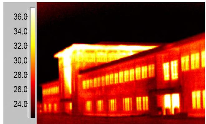
Image 11: During the commissioning of this building thermography revealed an extreme problem involving exfiltration through the soffit. Courtesy Phil McMullen.
