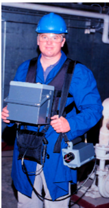
The author using a modern $60,000, cryogenically-cooled, "portable" IR system in the early 1990s.
