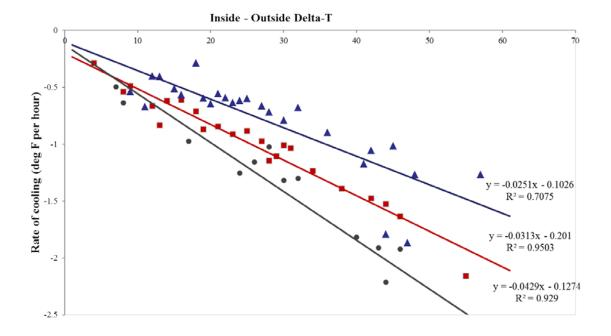
Figure 7: Degrees difference between inside and outside versus rate of cooling
